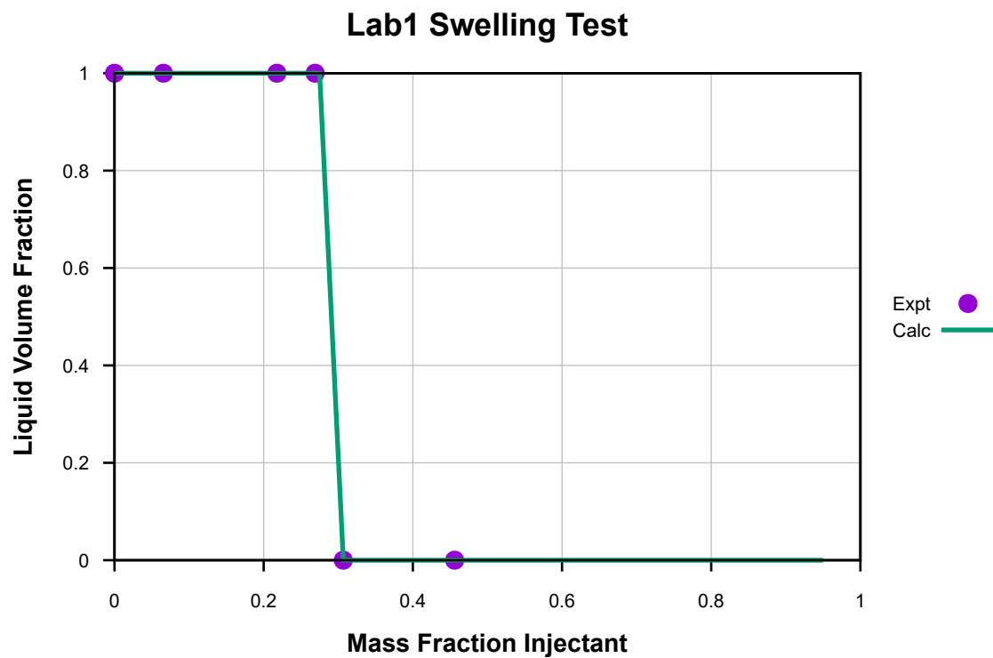
Figure 13: Liquid Volume Fraction vs. Mass Fraction Injectant for Lab1 Swelling Test.
